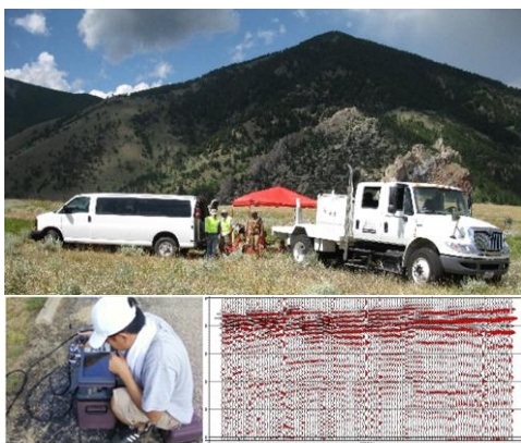
Left to right from the top: AGL field team at Montana, testing with StrataVisor NZ, VSP results (edited using Gedco Vista).
